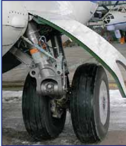
An-148 landing gear of BT-22 alloy
