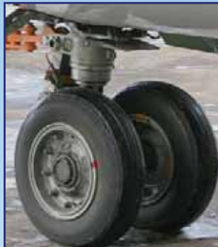
An-148 landing gear of BT-22 alloy
